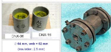
Fig. 1: inhibited FOX-7/GAP propellant grains DNX-06 and DNX-16 prepared to be tested in Ø 70 mm rocket motor
