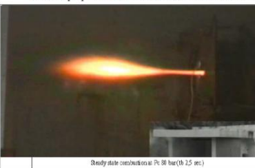
Fig. 2: Plume signature of a static motor firing with minimum-smoke DNX-06 propellant FOX-7/GAP/AP composition
