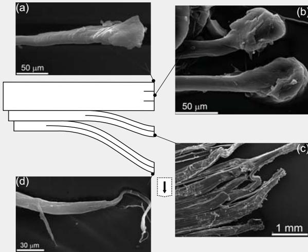
Micrographs showing the evolution of fibre fracture throughout the penetration cavity of a 35 mm thick target impacted by 12.7 mm FSP.
