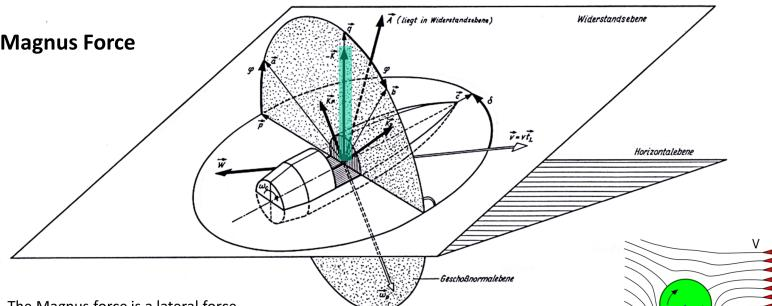
The Magnus force is a lateral force acting on a spinning projectile with a non-zero angle of repose as result of friction at the boundary layer of the air flow.
