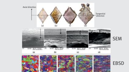
Fragments were soft-caught and analysed with regard to the fracture surfaces and deformation using SEM and electron backscatter diffraction (EBSD).
