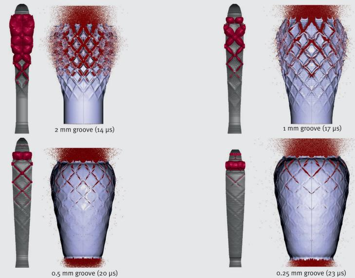
Numerical simulation of the deformation and breakup of the casing. For each groove depth, LS-Dyna to the left and Impetus to the right
