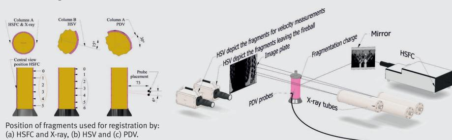
Position of fragments used for registration by: (a) HSFC and X-ray, (b) HSV and (c) PDV.
