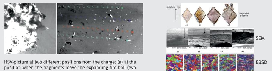
HSV-picture at two different positions from the charge: (a) at the position when the fragments leave the expanding fire ball (two fragments are marked with circles) and (b) at 1.2-1.5 m from the charge were the terminal velocity of the four leading fragments are evaluated. The direction of flight is to the right in the pictures.
