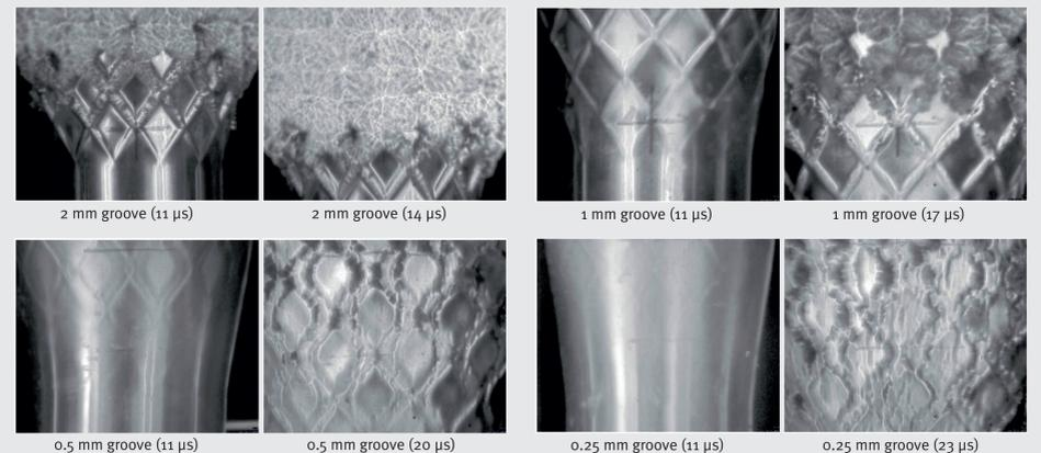
HSFC-pictures showing the initial deformation pattern of the casing at two different times. Left, arrival of detonation front. Right, start of fragmentation (matching the times of the numerical simulation snapshots shown above).
