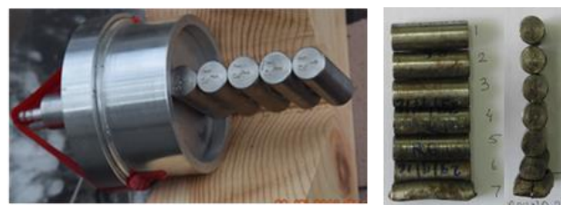
Figure 3: Test warhead and recovered fragments.
