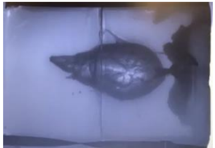
Figure 8: Temporary cavity formation across the gelatin blocks after projectile has passed through lungs
