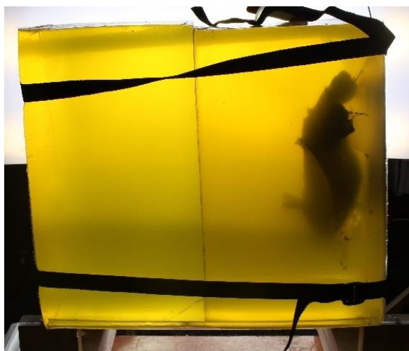
Figure 7: Lung model backed by plain gelatin block and strapped together
