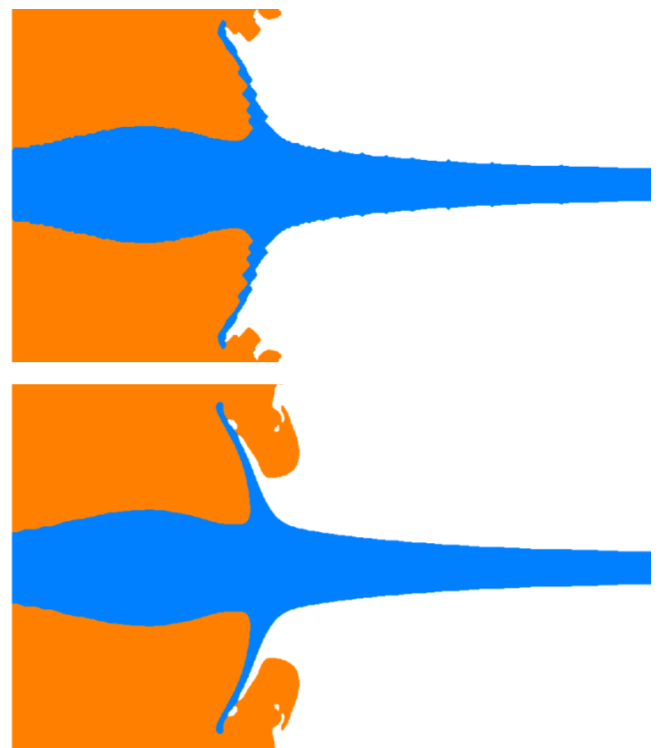
Figure 9: Zoom on the collapse zone of the shaped charge jet: simulation with SLIC (top) and PLIC (bottom)
