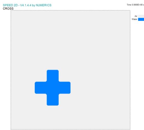
Figure 3: Initial position, velocity field ( v_x = 1 m/s, v_y = 1 m/s), 50 \times 50 grid
