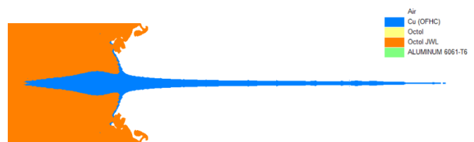
Figure 8: Shaped charge profile at t = 60 \mu s (SLIC method)
