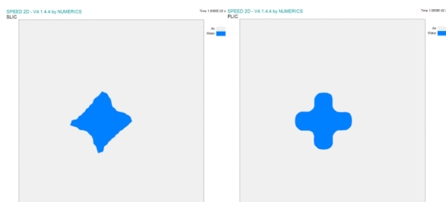
Figure 4: Comparison SLIC and PLIC results at t = 10 ms
