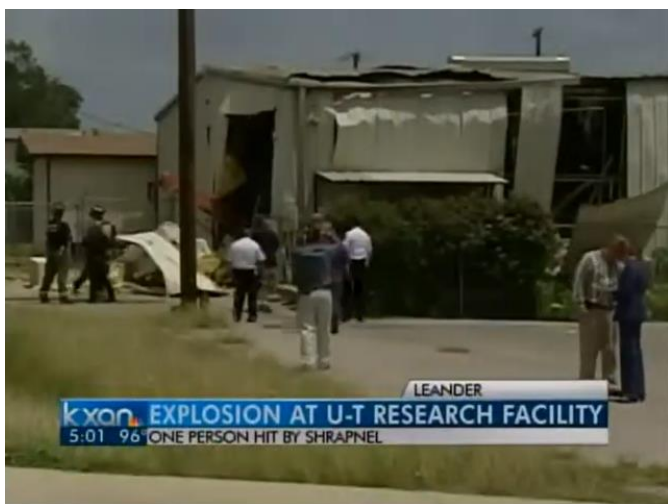
Figure 1: Video-news [2] of the accident at the UT light-gas gun in Leander on 12 June 2012. The damage to the metal-sheet housing resulted from both overpressure and accelerated gun components. A passing driver suffered minor injury.
