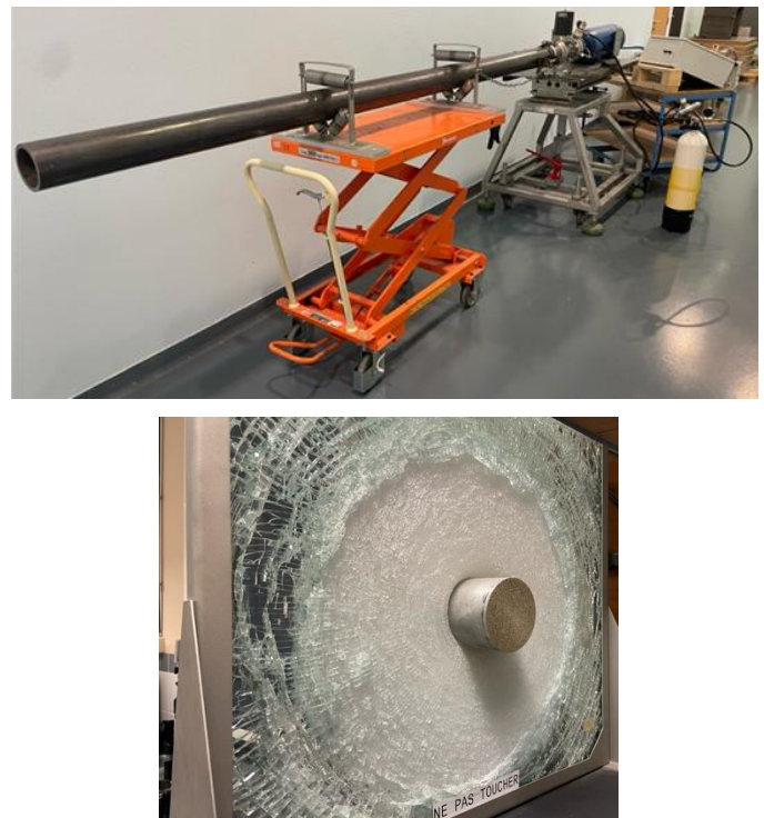
Figure 7. (Top) In-house pneumatic launcher developed for accelerating UIC projectiles – (Bottom) UIC projectile impacting the windscreen of a high-speed train.
