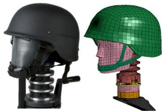
Figure 9. (Top) Testing ballistic protection and measuring the corresponding Back Face Signature – (Bottom) The Blunt Load Sensing Head-form (BLSH) wearing an helmet and its numerical twin for assessing Behind-Helmet Blunt Trauma.
