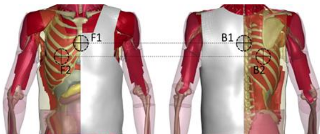
Figure 3: The GHBMCM50 model in cross-section with applied PPE and underlying tissue; (left) anterior with two impact zones: POI-F1 center of sternum, POI-F2 transition from 5 th rib to cartilage tissue; (right) posterior with opposing impact zones: POI-B1 center vertebra T7, POI-B2 between 9 th and 10 th rib.
