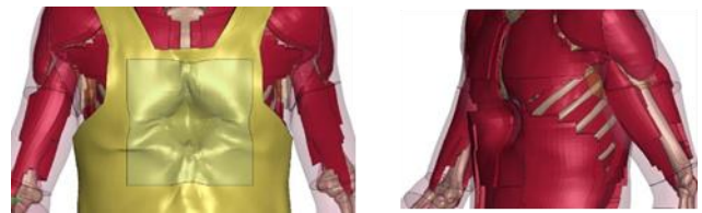
Figure 1: (left) Fabric pack on the GHBMCM50 chest at 1 ms; (right) back face deformation of the HBM.
