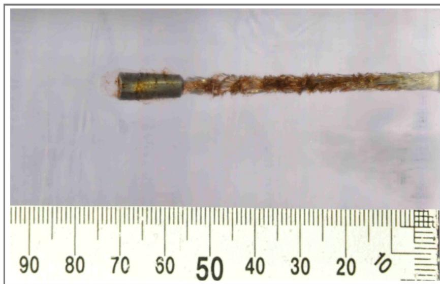
Figure 11. Deep penetration of 5 mm flat projectile in polycarbonate.
